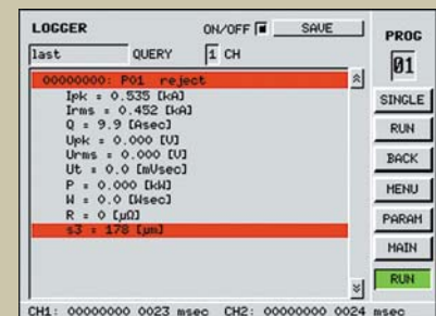
SPC Data Logger. All welds, rejects or last can be saved to the memory card.
